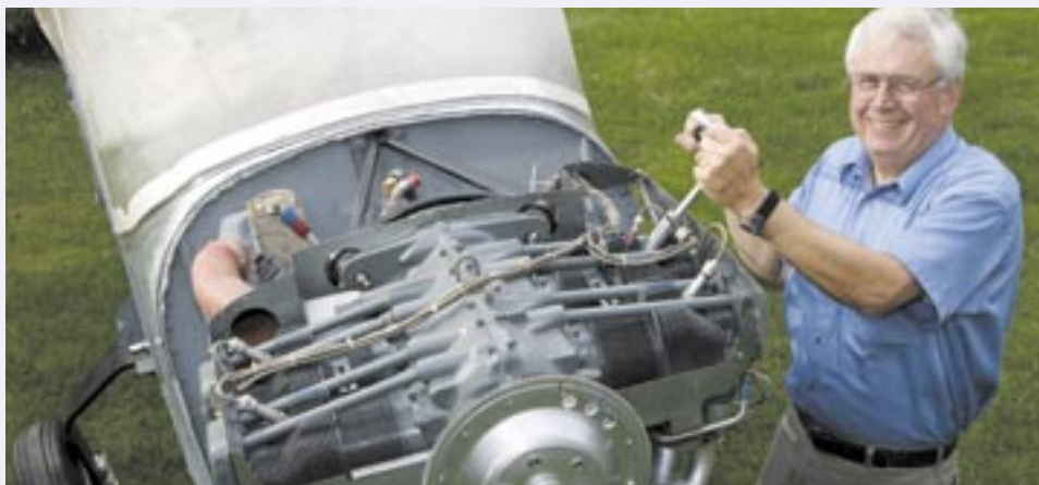
Rebuilding a 22-year-old, 180 HP Lycoming engine with only 245 hours of use took Dan an entire winter. It came intact from a plane wrecked by a tornado at Bradley International Airport.
