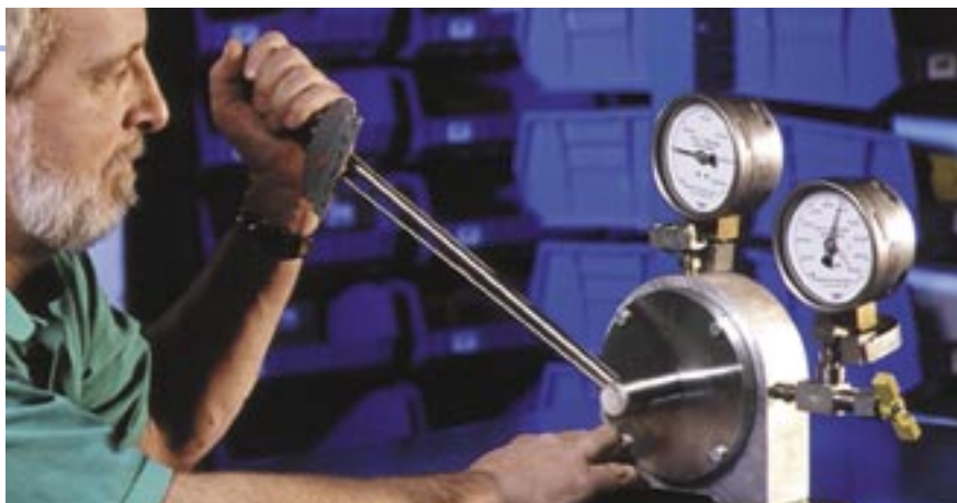
Using our Skidmore-Wilhelm tester, mechanical engineer Don Mahall will help you determine the amount of torque required to achieve a specified bolt tension.
